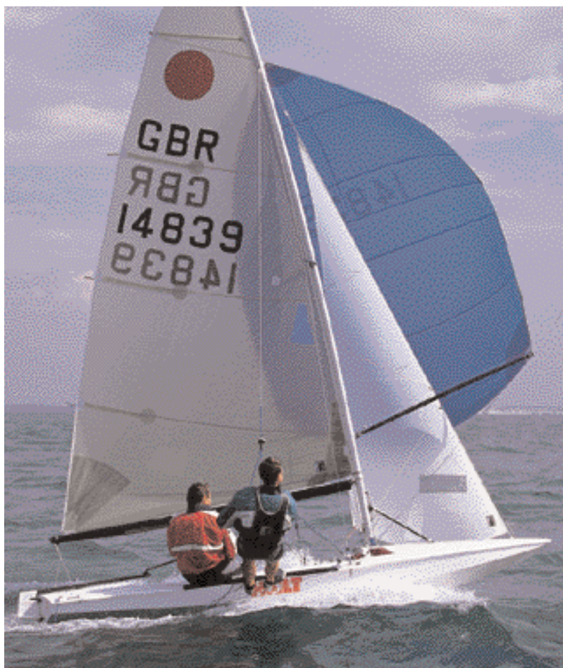
Above A Fireball can point higher than many asymmetrics with its asymmetric kite on a shy reach - the kite is stable with full vertical and horizontal adjustment for the pole.
